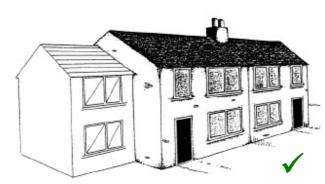
An extension is best designed to be subordinate to the existing building, i.e. not extending the full depth of the dwelling and should be set back from the front wall of the dwelling in recognition of its subordinate nature. Permitted development rights for ground floor extensions (up to 50% of the existing dwelling width) allow
