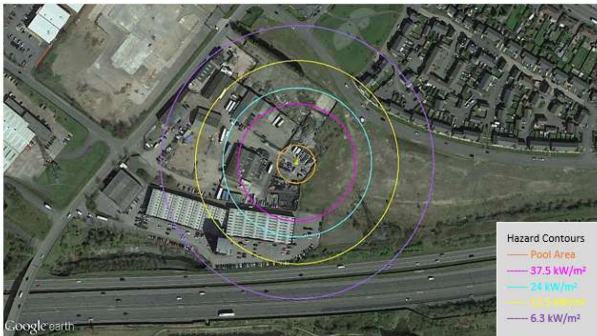
Figure 6 Butane Pool Fire Thermal Radiation Contours – F2 Weather
