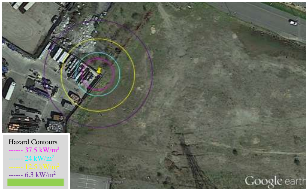
Figure 4 Pentane Pool Fire Thermal Radiation Contours – F2 Weather
