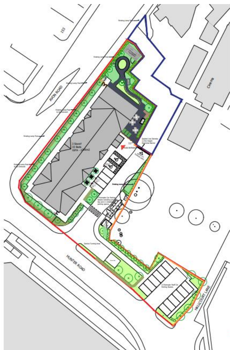
Figure 6: Proposed Site Plan Extract as amended showing two access locations onto Hunter Road
