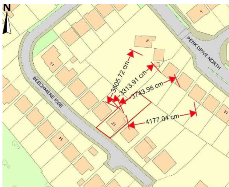
Figure 2: Extract from location plan shown scaled measurements to nearby properties taken from the facing edge of the balcony
