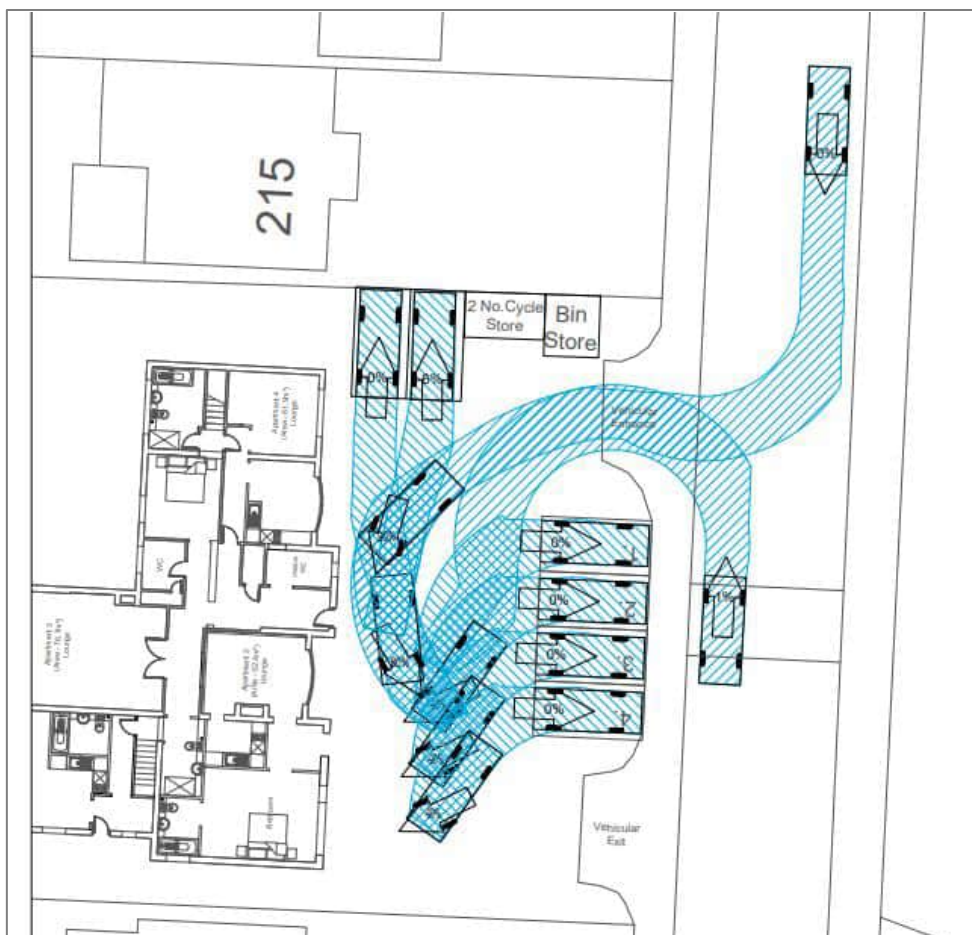
Figure 4: Imagery showing extract from Amended Parking Tracked path analysis. It should be noted that whilst cars about the front boundary, to reverse there still would be ample space for manoeuvring within the site curtilage.
