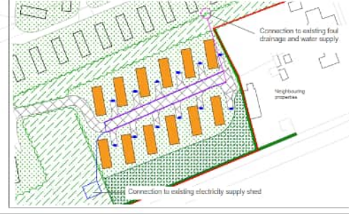
Plan of services (not to scale): All excavation to enable the installation of services within the trees/hedge/row areas to be hand dug to maximum depth of 500mm.
