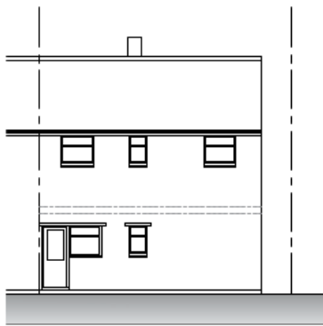
Existing Rear Elevation 1:100
