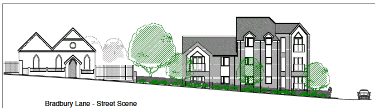
Fig showing the relationship between the proposed building and the converted chapel on Bradbury Lane.
