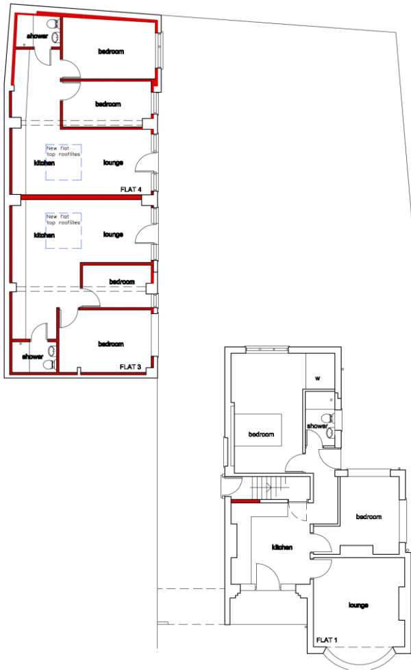
PROPOSED GROUND FLOOR PLAN 1:100
