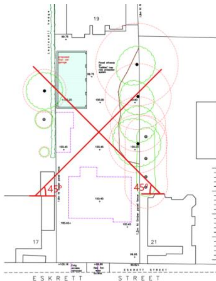
Figure 4: Imagery showing application of 45 degree standard lines
