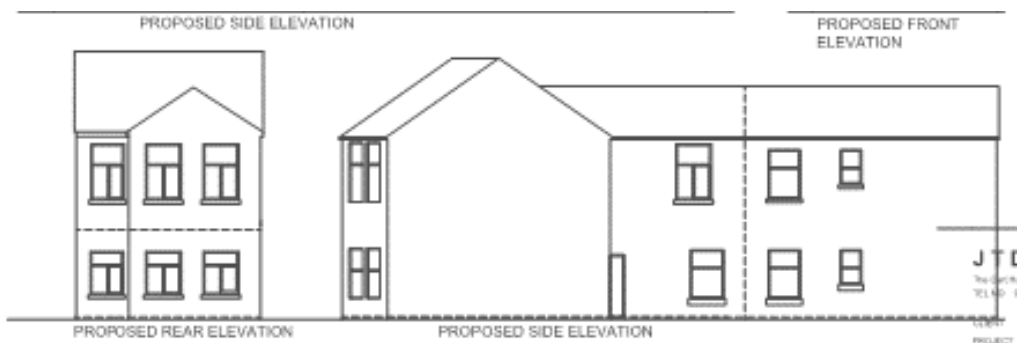
Figure 2: Extract from Proposed Elevations showing rear extension denoted by dotted line (right)
