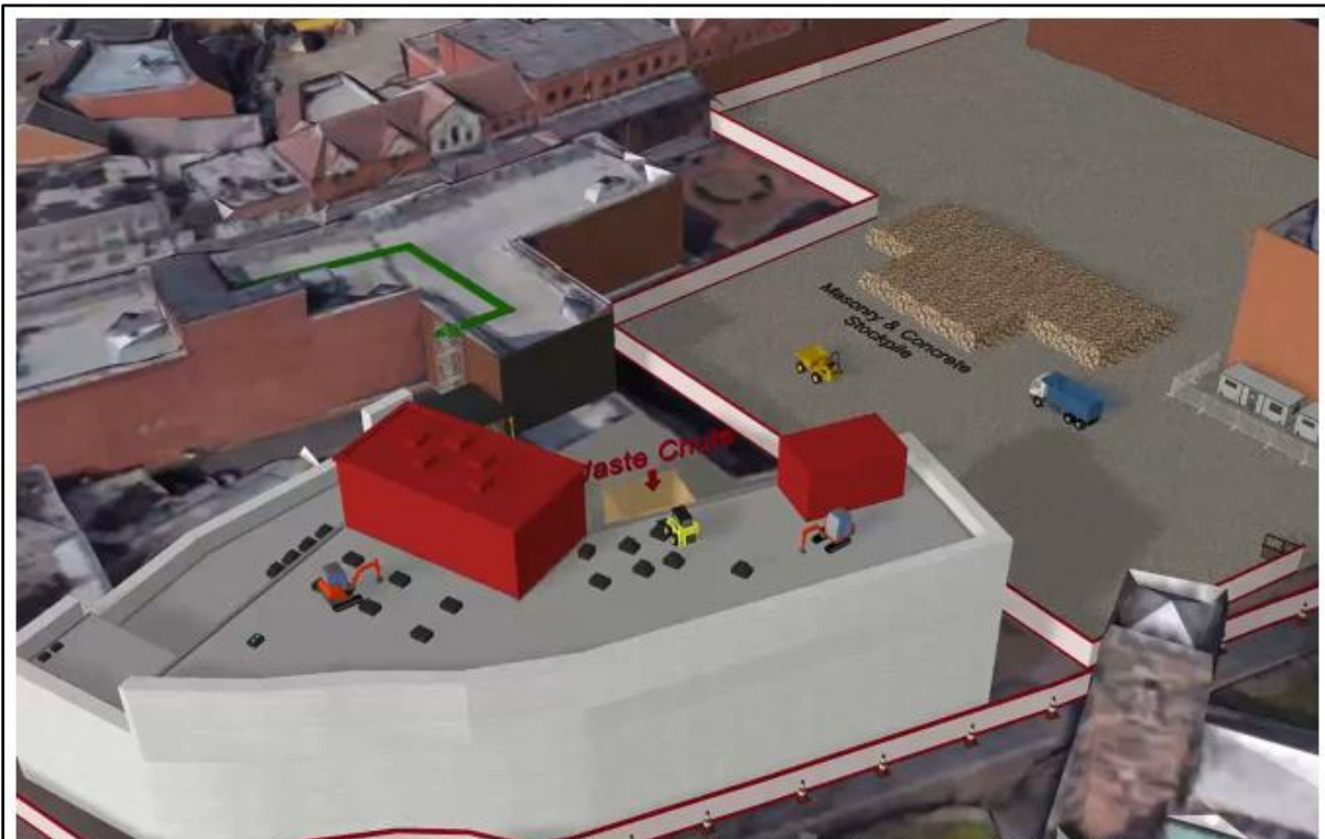
Waste Chute to be erected to enable waste to be removed to the rear of the building.
