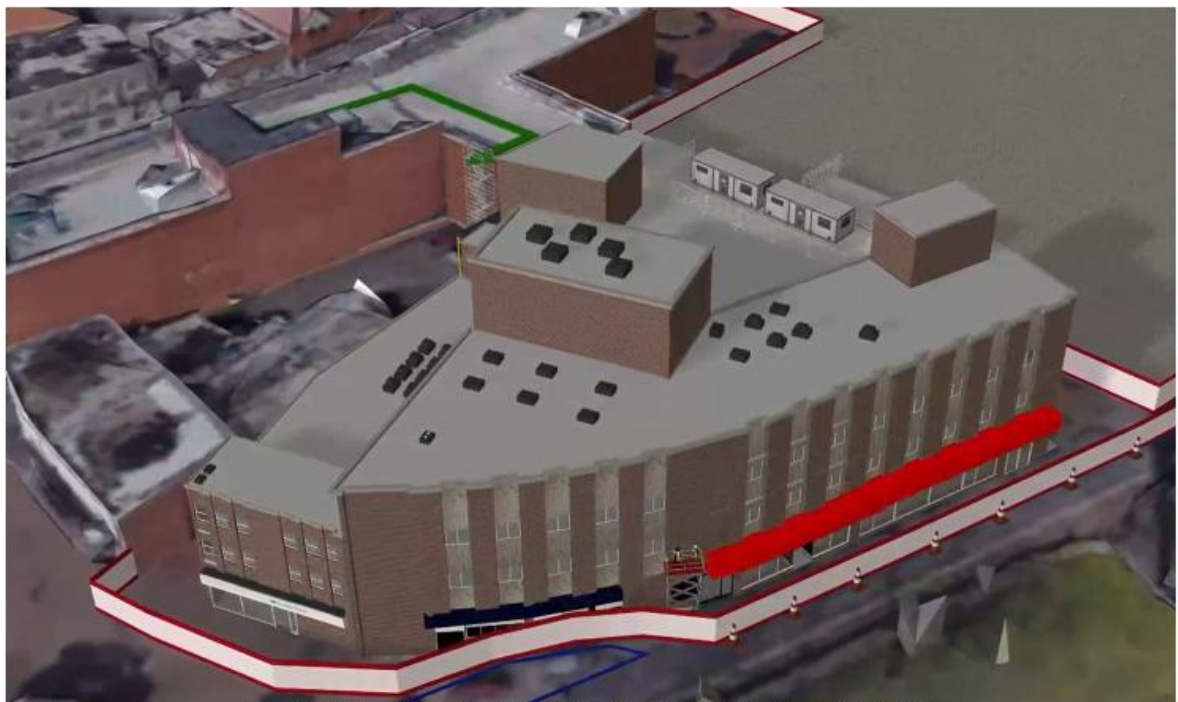
Front sections of the gantry to be demolished from inside the hoarding line.
