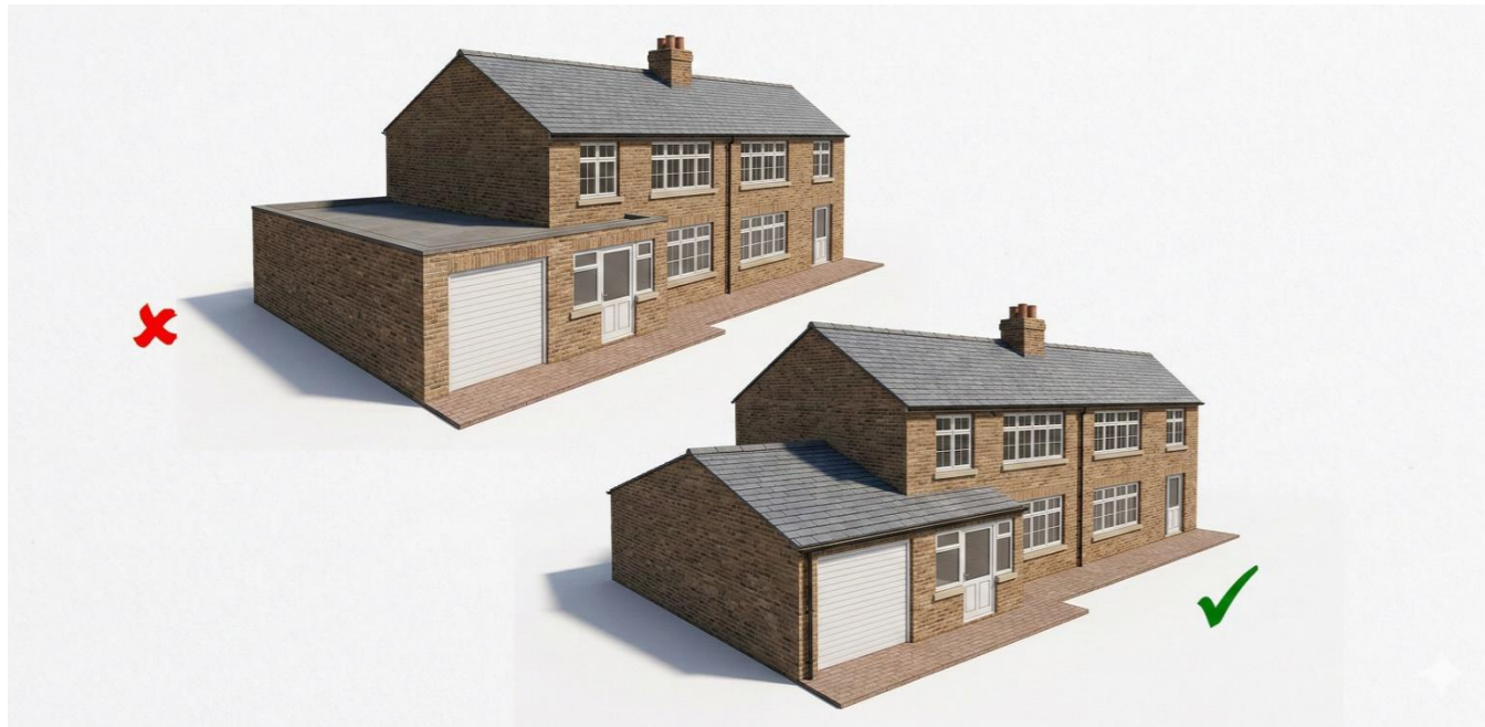
Figure 12: Extension reflects form of existing house
