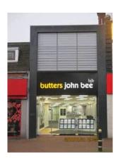
Security shutters – suitable options include internal to shop window, perforated and painted to match the shopfront
