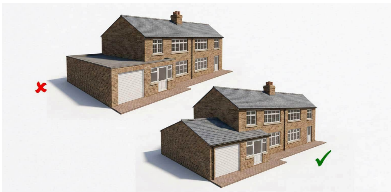
Figure 12: Extension reflects form of existing house
